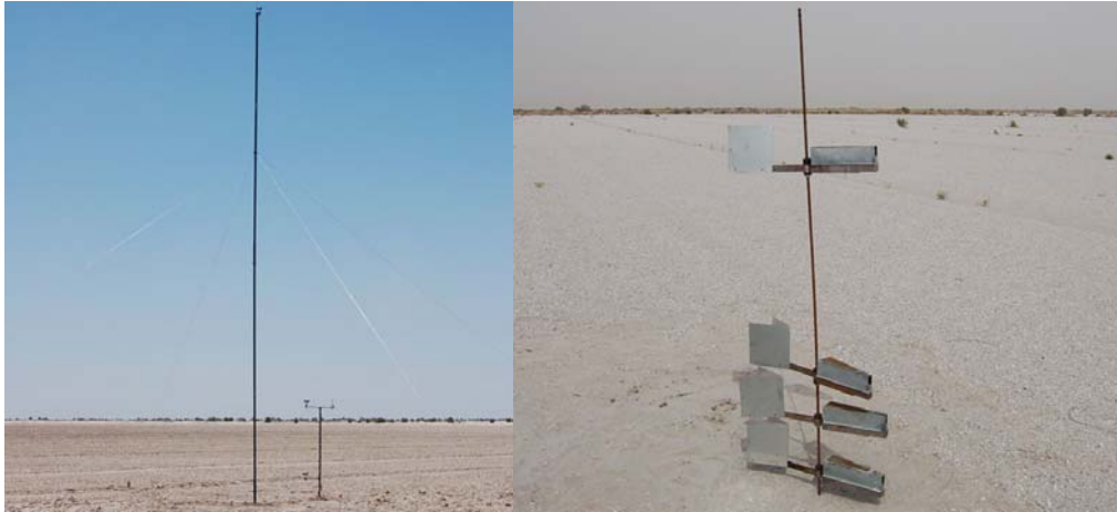
Fig. 3: Wind station and sand traps
