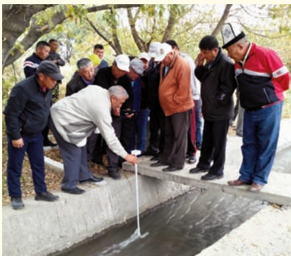
Figure 11: Mirabs in Kyrgyzstan testing the SmartStick device for measuring water levels
