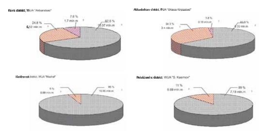
The percentage of collector-drainage water withdrawals from different sources within WUAs for vegetation 2008
