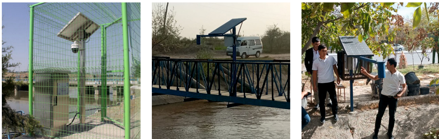
Figure 2. Automated Smart Water level sensors along irrigation canals
