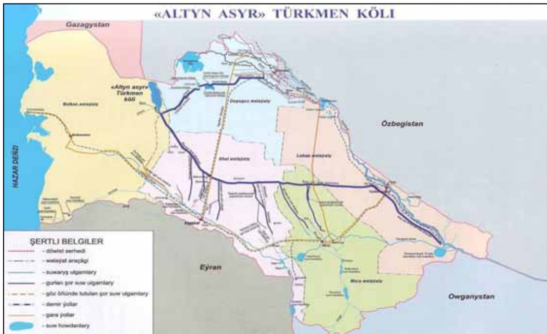
Fig.1. Layout of collectors transporting water to Lake Altyn Asyr
