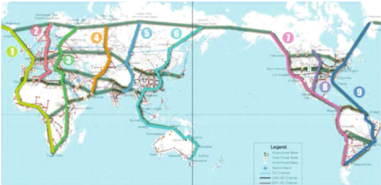
Backbone transmission lines of GEI (Global Energy Interconnection, GEIDCO 2018)
